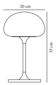
IP degree: IP44 Class (Class 1, Class 2, Class 3): Class 3 (12V) Socket type: LED Module
