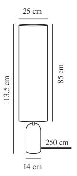
Voltage (V): 220-240 Volt IP degree: IP20 Maximum bulb wattage (W): 40W Class (Class 1, Class 2, Class 3): Class 2 (Double isolated) Socket type: E27 Switch placement: On the cable Parallel connection: False
