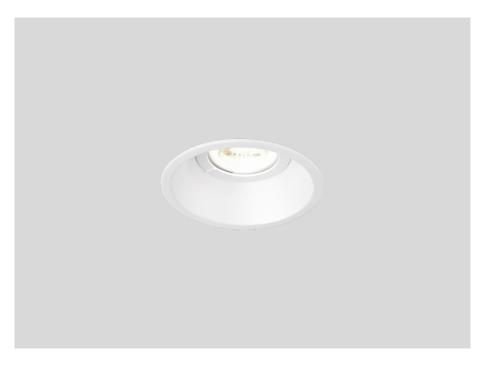
Round ceiling recessed downlight made from die-cast aluminium; surface Signal White; powder coated; matt texture; RAL 9003; installation without tools using wire springs; suitable for ceiling thickness of 4-25 mm; recessed depth 105 mm; lamp socket GU10; lamp type PAR16; max. 12W; 100 - 240 V; degree of protection IP44; PC2; UGR 16; VDU compatible workplace luminaire according to DIN EN 12464-1; luminance above  $65^{\circ}$  1500 cd/m²; lamp not included;
