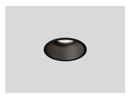
Round ceiling recessed downlight made from die-cast aluminium; surface Jet Black; powder coated; matt texture; RAL 9005; installation without tools using wire springs; suitable for ceiling thickness of 4-38 mm; recessed depth 115 mm; lamp socket GU10; lamp type PAR16; max. 12W; 100 - 240 V; degree of protection from below IP44; from above IP20; PC2; lamp not included;
