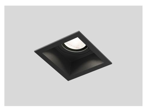
Squared ceiling recessed downlight made from die-cast aluminium; surface Jet Black; powder coated; matt texture; RAL 9005; installation without tools using wire springs; suitable for ceiling thickness of 4-30 mm; recessed depth 115 mm; lamp socket GU10; lamp type PAR16; max. 12W; 100 - 240 V; degree of protection from below IP44; from above IP20; PC2; lamp not included;
