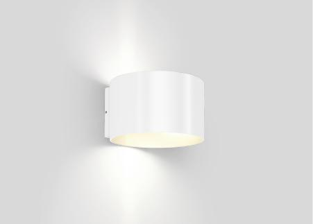
Cylindrical wall surface mounted luminaire made from aluminium; surface White Matt; powder coated; matt texture; RAL 9010; direct/indirect light distribution; lamp socket G9; lamp type QT14; max. 75W; 220 - 240 V; degree of protection IP20; PC1;
