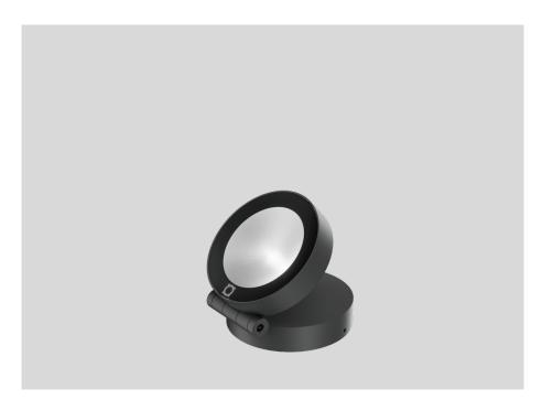
Round outdoor floor or wall projector; surface Anthracite Grey; powder coated; matt texture; RAL 7016; with COB (Chip on Board) technology for maximum efficiency; phase-cut dim; light colour 3000 K; binning initial MacAdam  $\leq$  3 SDCM; CRI  $\geq$  80; 220 - 240 V; 110° tiltable; beam angle 108°; degree of protection IP65; PC2; driver included; optional ground spike available; optional snoot in Black Matt available;
