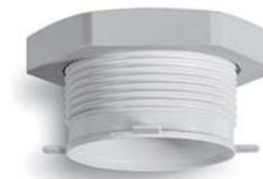
The easiest way to flush-mount elements from our DOT 28 system into drywall is to use our SPACKLING RING. Drill hole into ceiling, screw in spackling ring, secure from back side, thread cable and go ahead with plastering!
