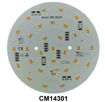
TypeLED moduleLamp wattage [W]3 WInput voltage [V]12 VDCEnergy classEFlux [Im]390 ImLight colour [K]2700 KCRI93Dimmableyes
